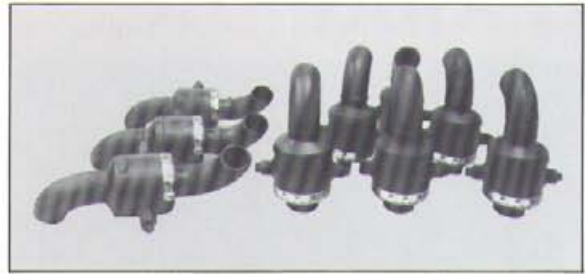
2" Series "S2" Style 30 and 40 Ball Joints designed for 1700 PSIG/650° F for installation in enhanced oil recovery piping. A total of 137 Ball Joints were furnished in 1½", 2" and 2½" sizes for Chevron Oil, Bakersfield, California.
