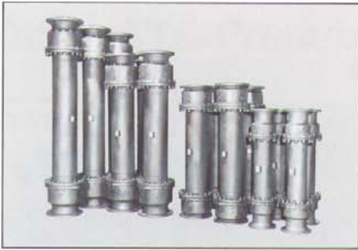
Six 16", four 14" and four 10" 150 lb. Flanged Series "S1" Ball Joint linkage assemblies to accommodate tank settling at the Yanbu Power and Desalination Plant in Saudi Arabia.
