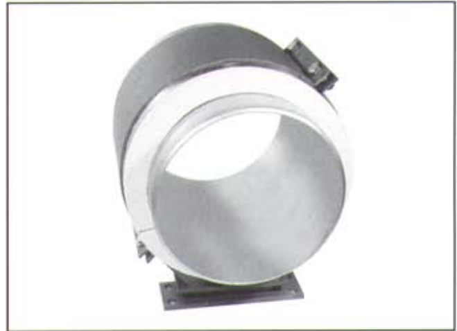
18" Fig. 201M-B-2-8-3 Pre-Insulated Pipe Support with 2" Thick Calcium Silicate Insulation and 0.016 Embossed Aluminum Jacket with Integral Moisture Barrier Split Line at 45° to permit Pipe Nesting
