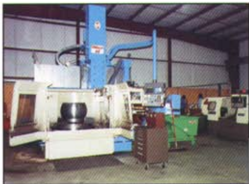
Modern machining facilities allows consistent close tolerances. 59" diam. CNC shown is one of three CNC's used for in-house machining of all components of the TP2 Expansion Joint and Flexible Ball Joints.
